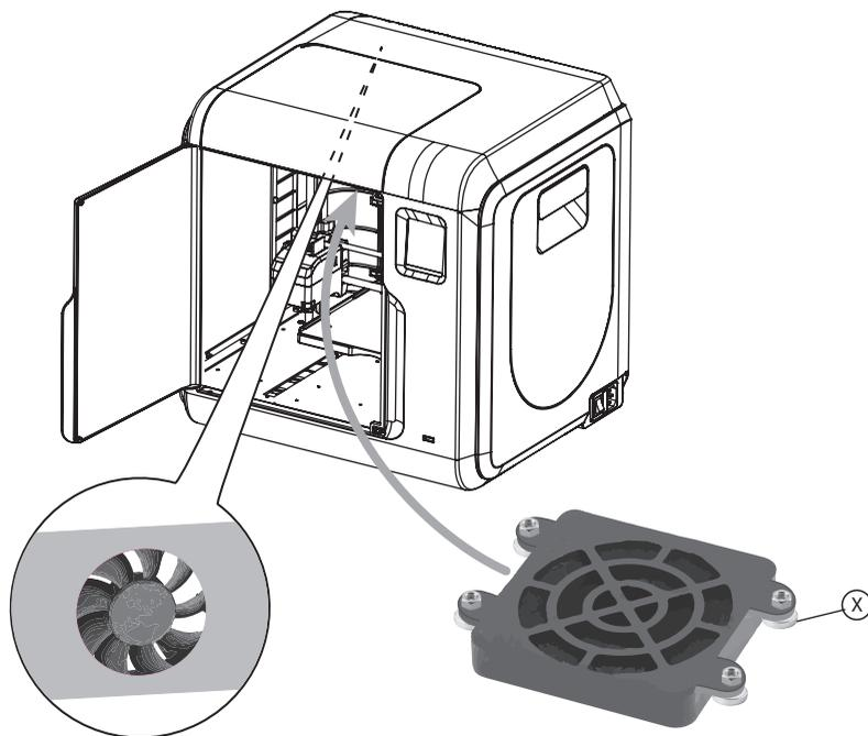
The printer is equipped with a fan located in the rear of the printer under the top cover. It is surrounded by a metal plate.
