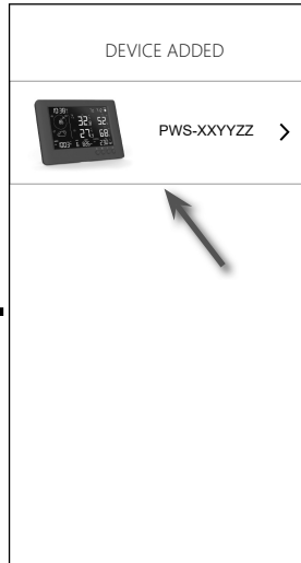
(e) Once the console is added to WSLink, the console icon will appear on your device list. Tap it to continue the setup.
